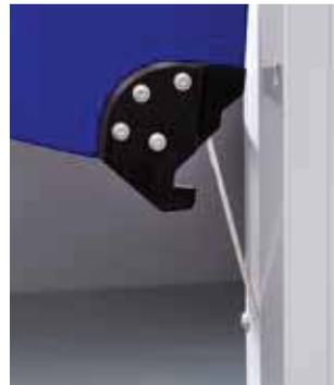
*In case of a collision, the closing edge can bend in all directions. Pre-stressed ropes ensure a controlled deformation until the snap-in connections between the edge of the door leaf and the guide pieces disconnect. Subsequently, the door curtain can slip out of the door frame guides in any direction.*
