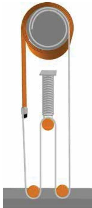
*The EFAFLEX wind load system provides permanent door leaf tension. Perfect where wind or negative pressure causes a draft!*
