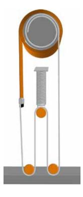
The EFAFLEX wind load system provides permanent door leaf tension. Perfect where wind or negative pressure causes a draft!
